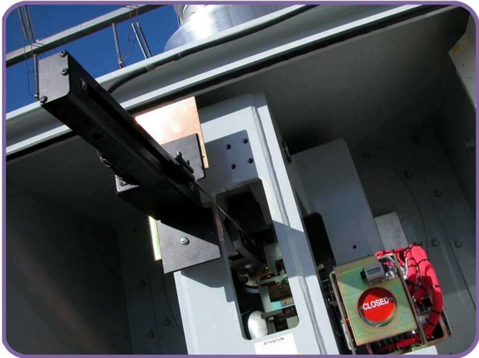
Figure 33. Linear Transducer on Mitsubishi 500-SFMT
